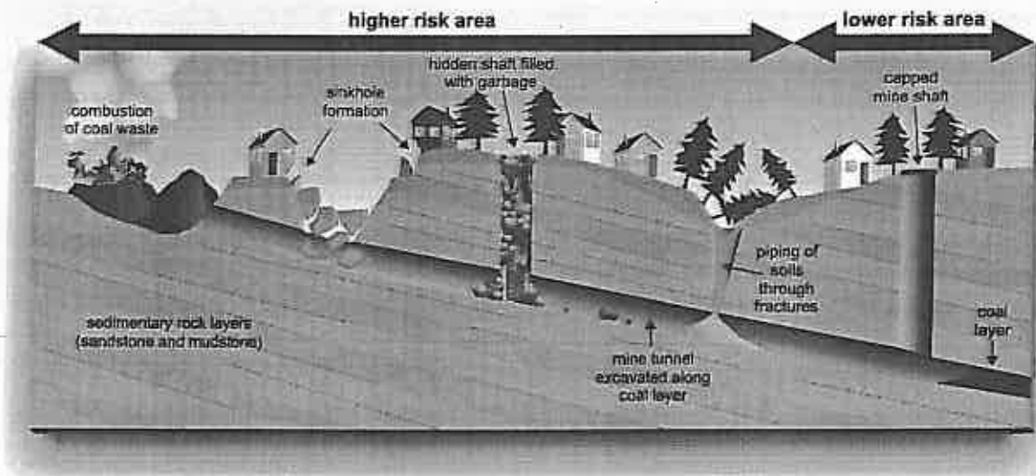
Illustration of mining related subsidence potentials (geoscape.nrcan.gc.ca)
